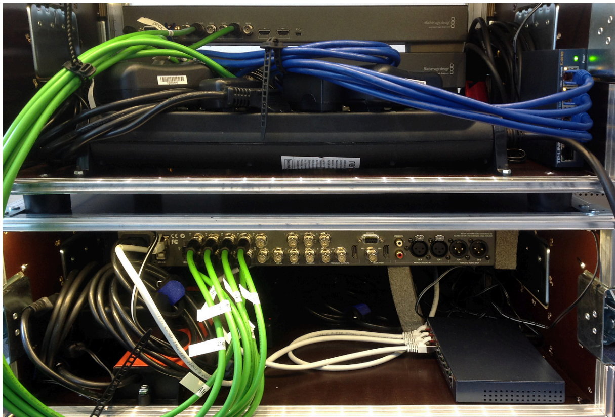
Example connection of multiple HyperDecks with an ATEM vision mixer (green cables) and a LAN network (blue cables)
